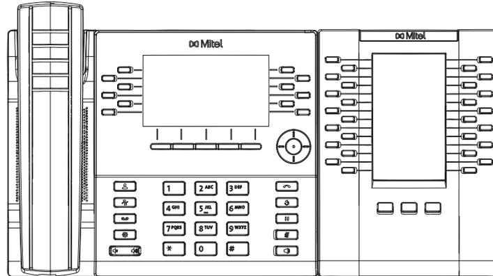
The Mitel M695 PKM features a 4.3" 480x272 pixel color backlit LCD display that provides a unified graphical user experience with the Mitel MiVoice 6930 IP phone.
